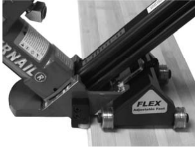
Figure 3. Raise the nailer foot to leave a small gap between the 2 small rollers and the flooring tongue.
