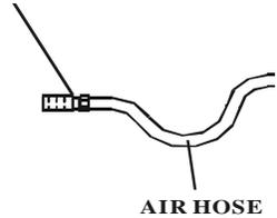
1. An automatic airline oiler is recommended but oil may be added manually before every operation or after about 1 hour of continuous use.
